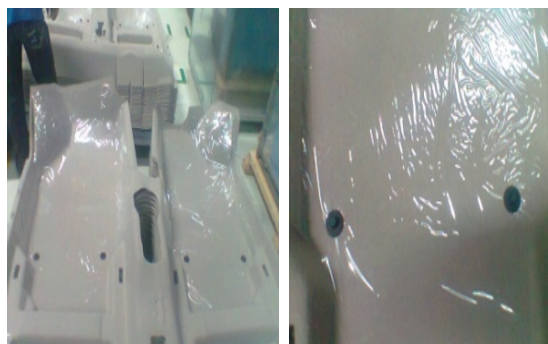
Fig. 1: Car Carpet showing holes and lock buttons
